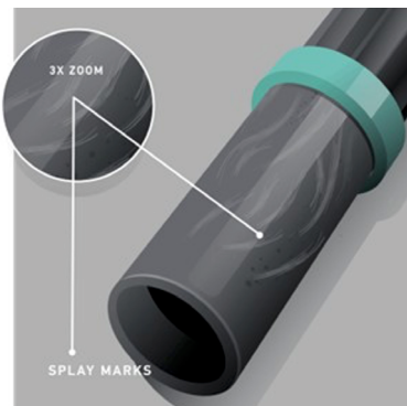
Splay marks on an injection-molded surface are typically caused by moisture or other volatiles flashing into gas during filling. Courtesy of Elastron.
