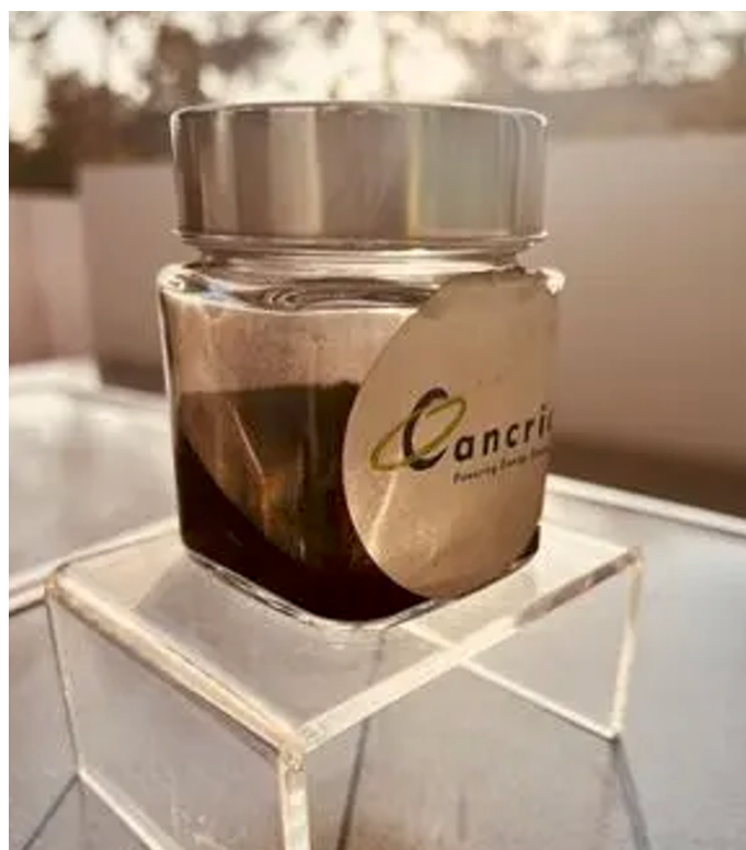
Nano-carbons produced by Cancrie from coconut shells, kernels, sugarcane bagasse, and hair waste
