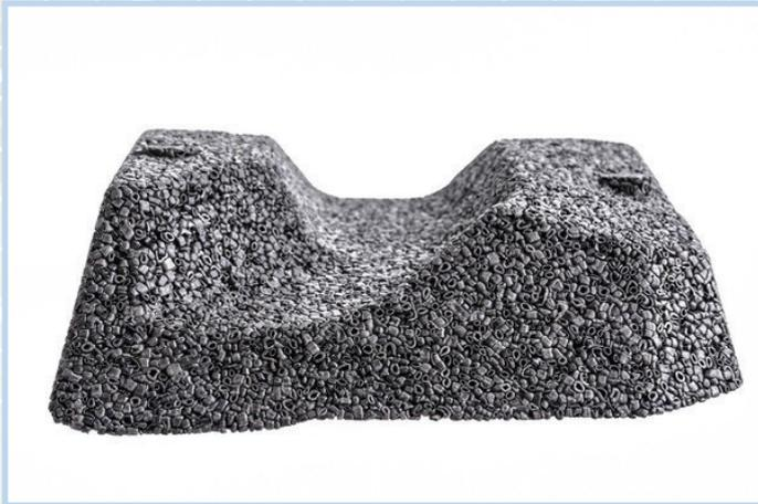
erations in the material, homes, and health care business announces the development of the PA Foam, a foam bead material based on polyamide – the first of its kind worldwide. This foam bead is considered to be perfect for noise reduction and lightweight applications in the automotive industry. The company is one of only four fully integrated polyamide manufacturers worldwide and is able to produce PA 6.6 completely from monomer to compound.
