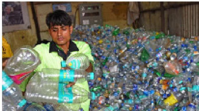
Currently, only PET, HDPE, and PVC plastic products are recycled under curbside recycling programs. PS, PP, and LDPE typically are not recycled because these plastic materials get stuck in the sorting equipment in recycling facil-
