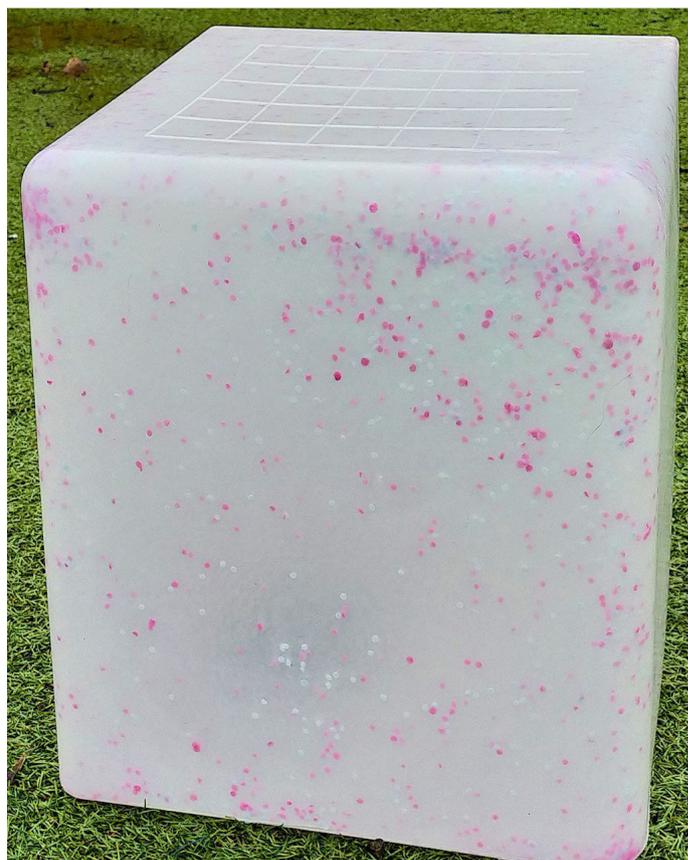
We are also thinking about the aesthetics of the blocks. Blends of recycled mixed-colour plastics usually end up with a grey or black colour. To enable colour, we are preparing blends of virgin or recycled plastics to overlay the main bulk of the block.
